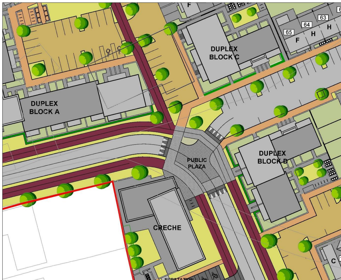
Figure 26: Excerpt from site plan showing proposed public plaza, shared surfaces, public spaces and raised table
