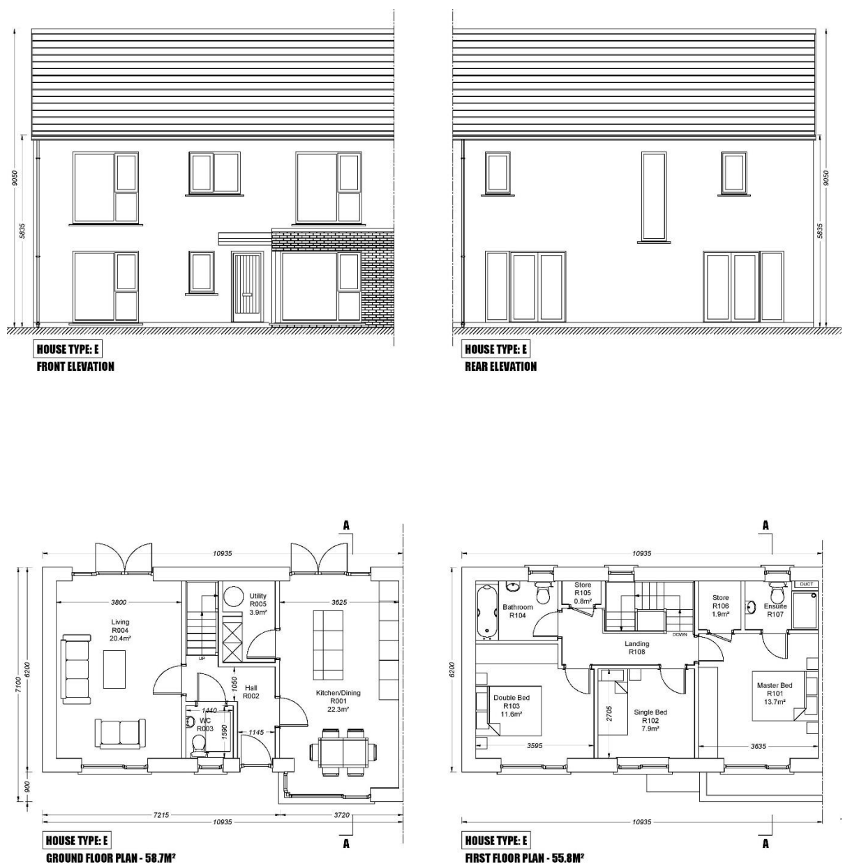
Figure 19: Type E house type, wide fronted house with all habitable rooms facing south.
